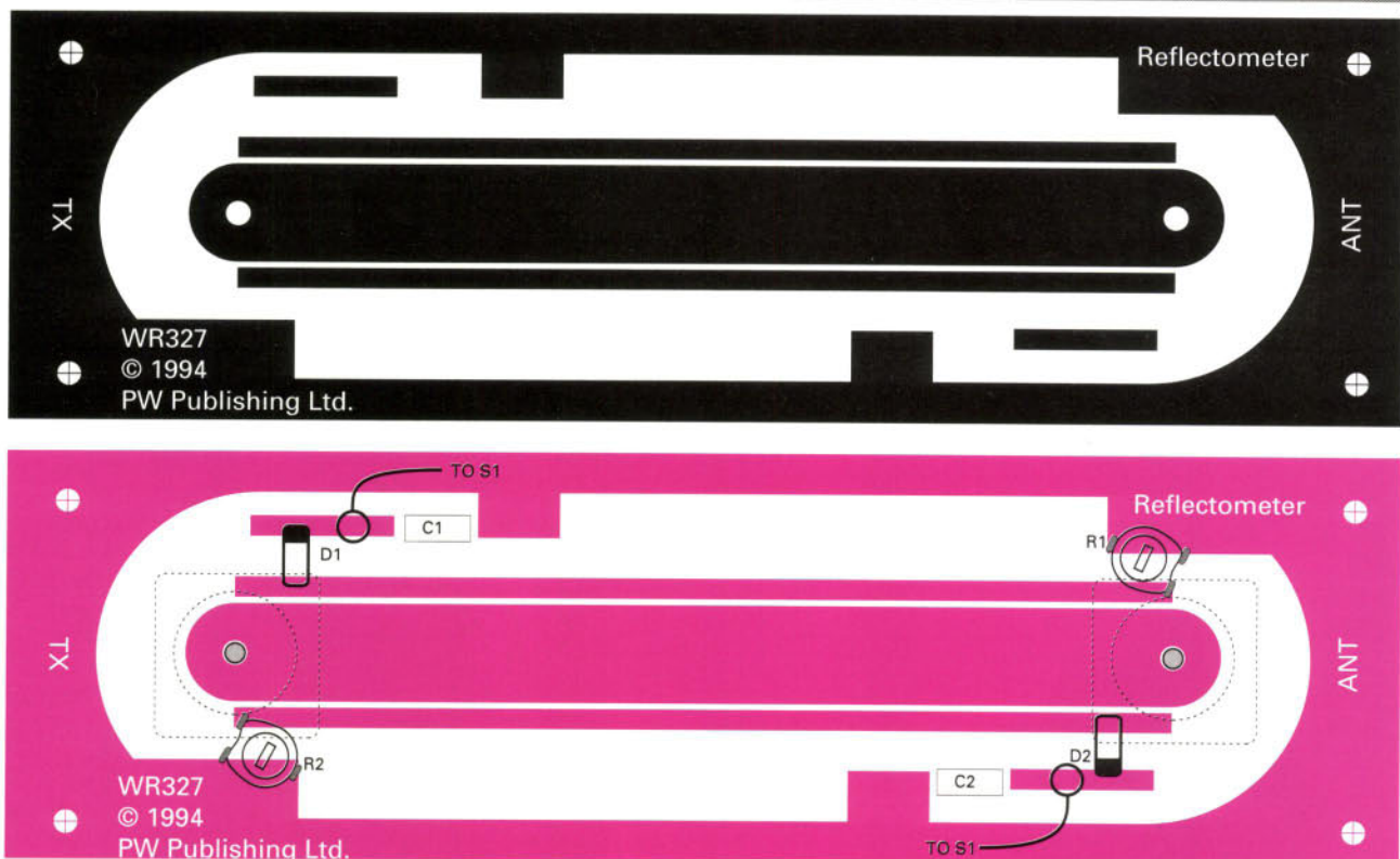
Fig. 2: Printed circuit board layout for the simple reflectometer. The few components are soldered into place using 'surface mount' techniques (see text).
